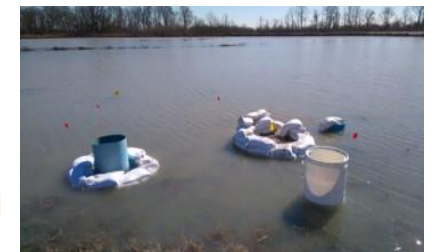
Figure 1: use of barrels to contain the wells
