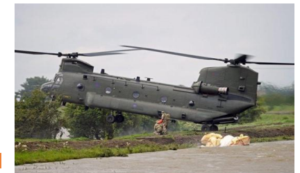
Figure 1: Chinook is used to close a breach using big bags, Wainfleet 2019
