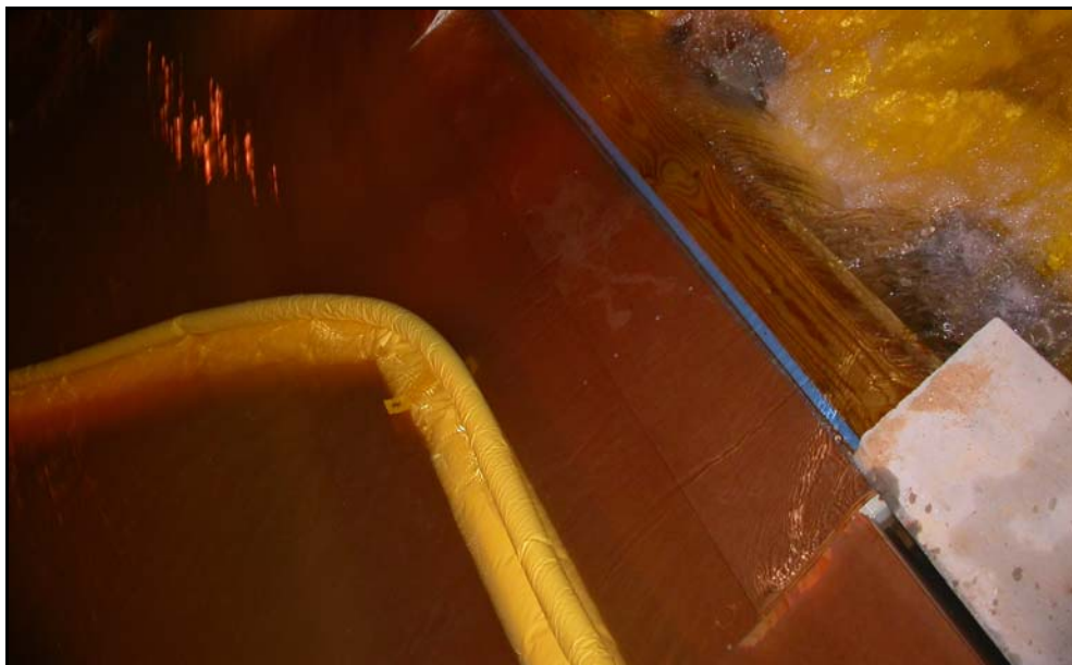
Figure 12. Shallow-water breach bag being carried into place by current.
