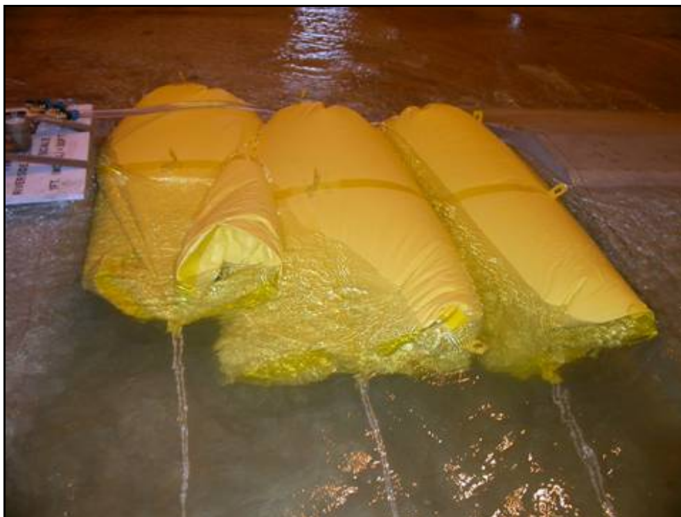
Figure 9. 30-ft-diam bags in breach, looking downstream.
