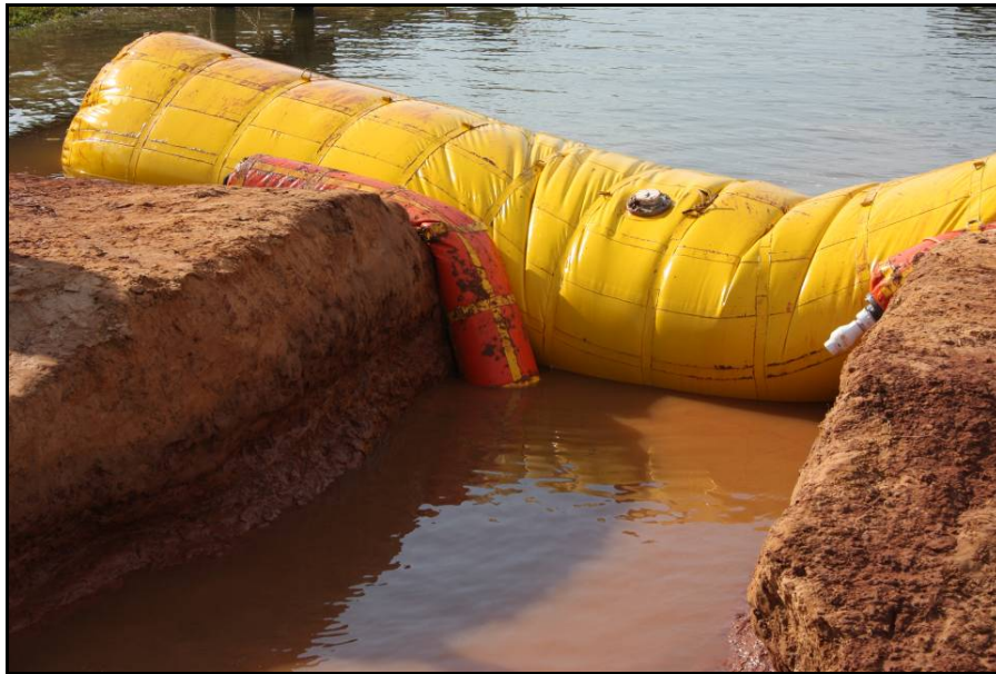
Figure 7.7. Sample deployment of deep-breach closure system including the addition of two small tubes along the upper edges of the breach opening which produced essentially zero-flow conditions through the breach.
