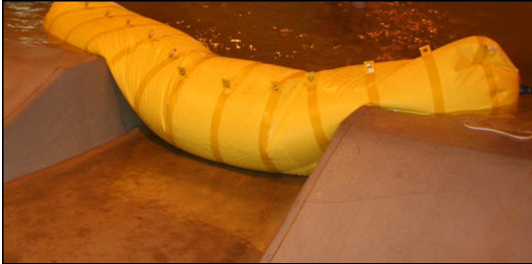
Figure 6.5. Deep-breach closure with large tube filled to 60% fill volume.
