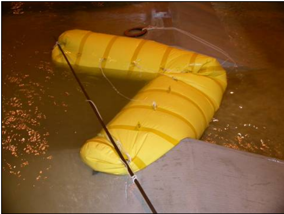
Figure 6. Beam and ties used to force 195-ft-long bag into a wedge shape.
