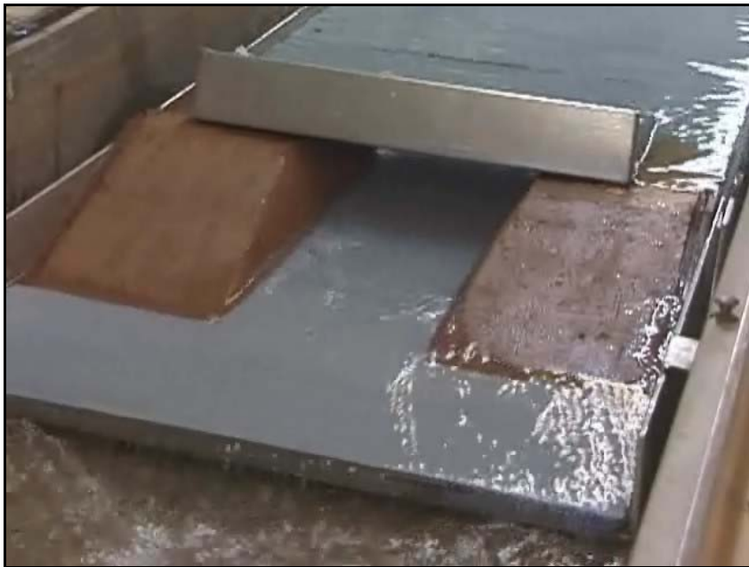
Figure 5.4. Idealized barge floated into position on small-scale levee and ballasted with water.
