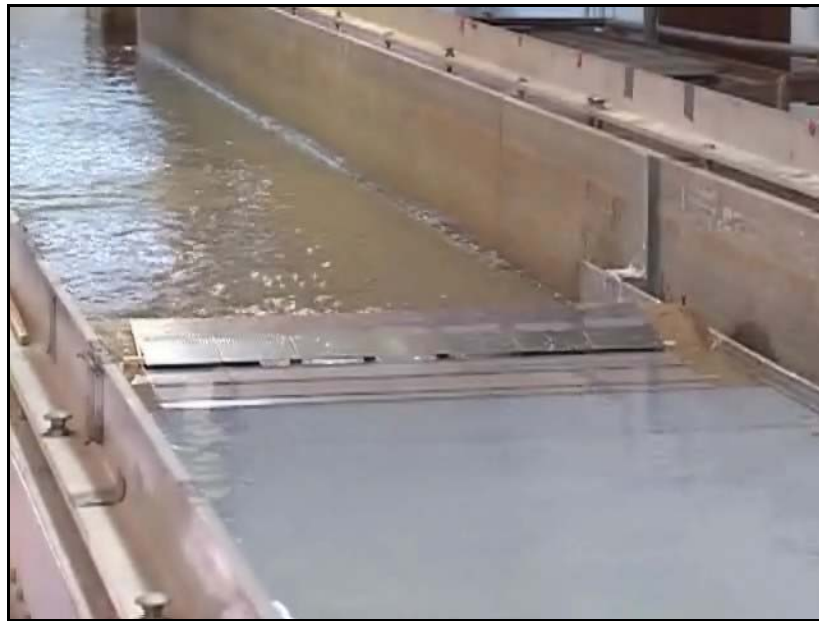
Figure 5.2. Photo of gated structure test in 1:50 scale flume.
