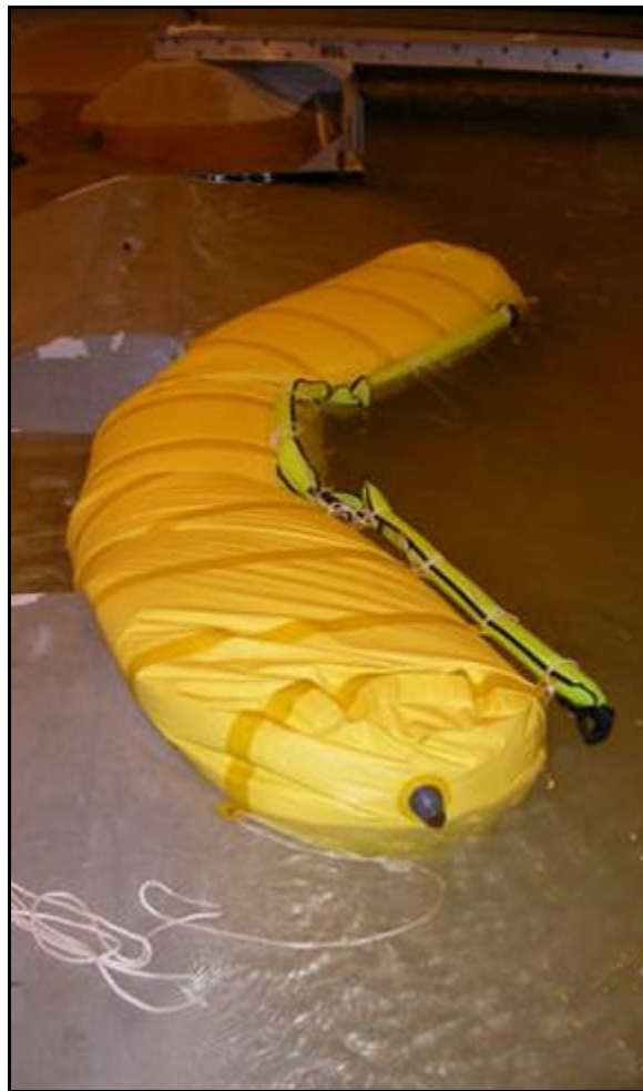
Figure 5. 195-ft-long bag deployed with outside air chamber.
