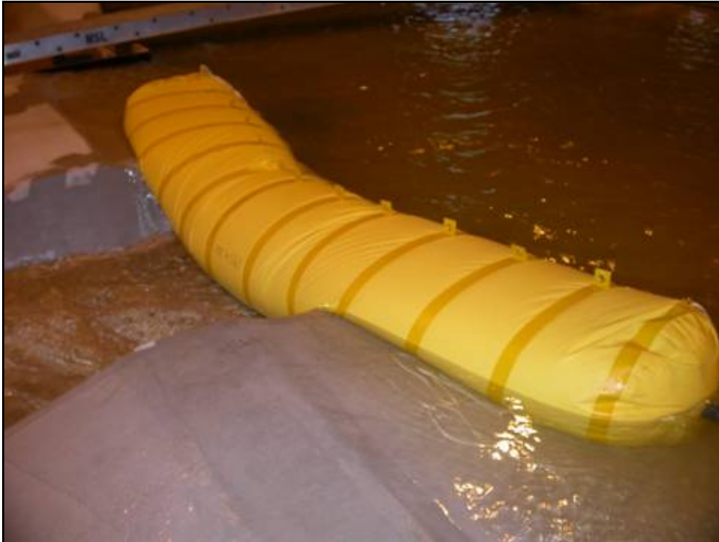
Figure 3. Breach sealed with 195-ft-long bag with 80% fill.
