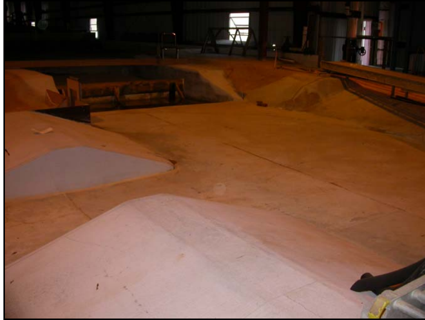
Figure 6.1. Test basin for 1:16 scale physical model tests.
