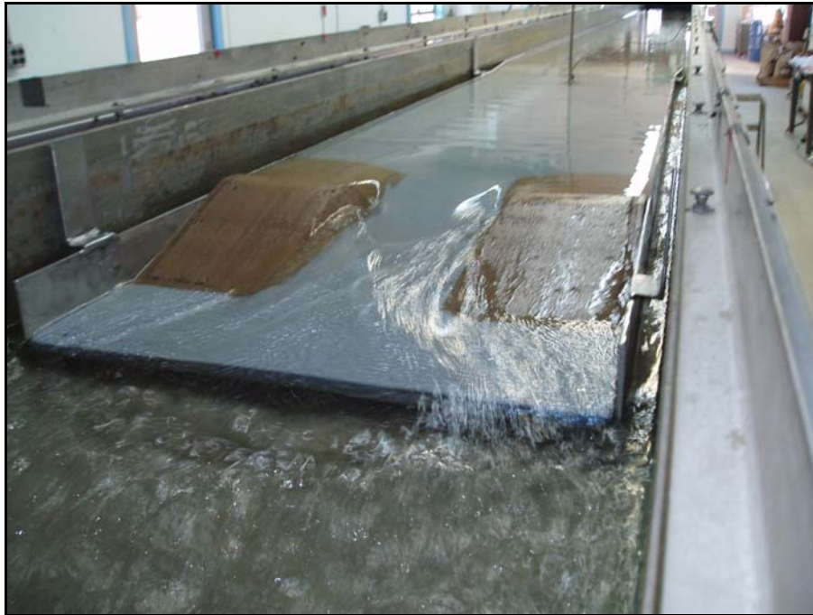
Figure 5.1. Photo of flow through small-scale (1:50) breach.
