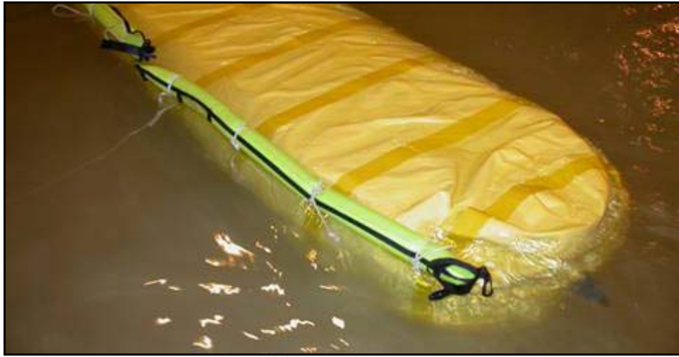
Figure 4. SCUBA signal tubes fastened along 195-ft-long bag.
