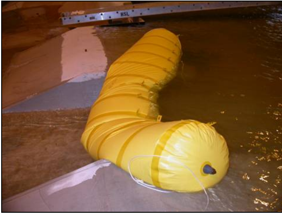
Figure 5. Breach filled with 195-ft-long bag with 65% fill and air left in bag before filling.
