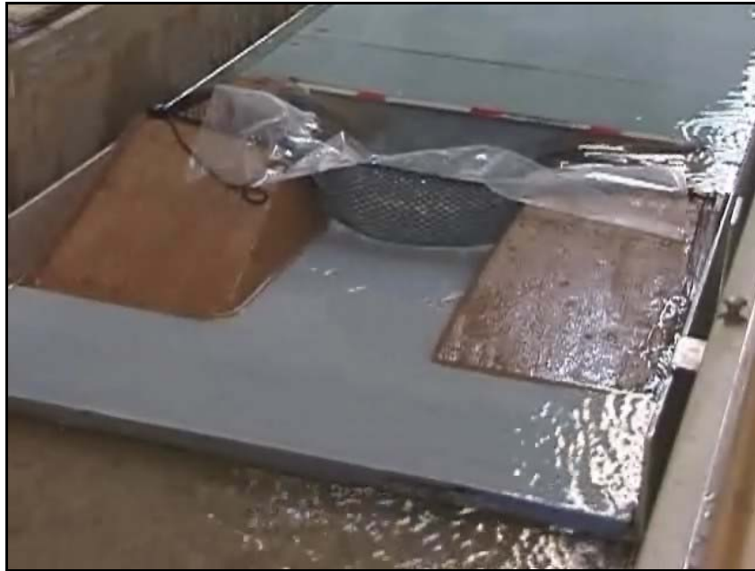
Figure 5.5. Photo of performance of a net anchored on either side of a breach combined with a tarp in the 1:50 scale model.
