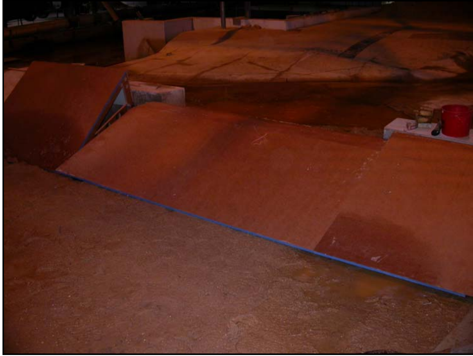
Figure 10. Plywood sections used to construct the shallow-water breach. The section on the left end is elevated only to illustrate the construction.
