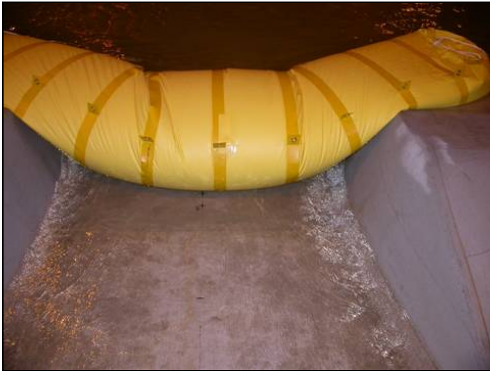
Figure 2. Breach sealed by 195-ft-long bag with 70% fill.
