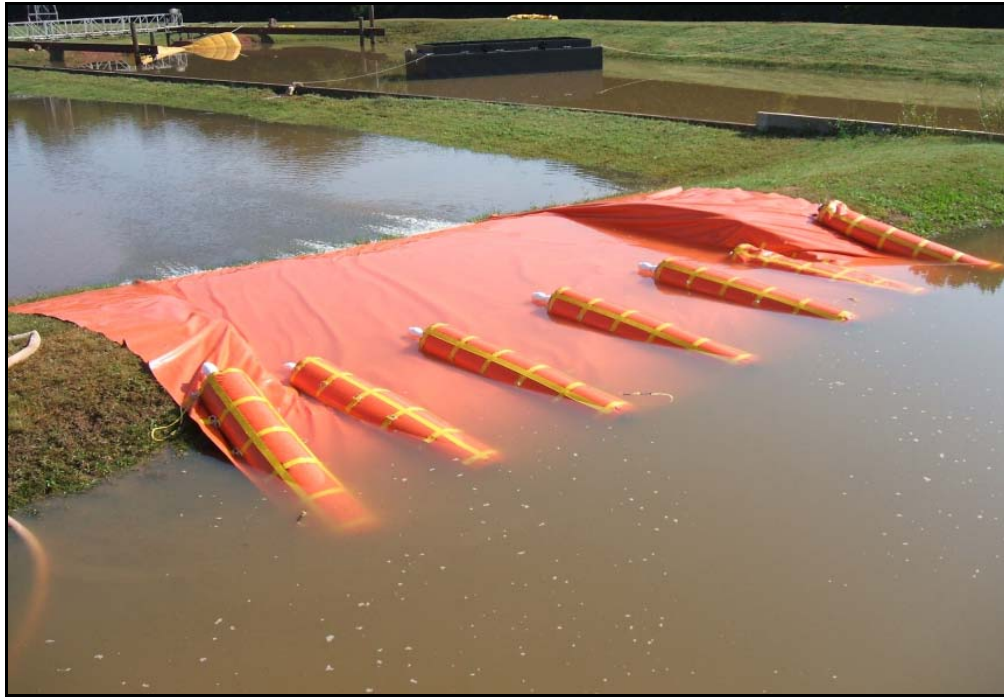
Figure 7.2. Demonstration of REPEL system with 0.5-ft of water passing over the top of the breach.
