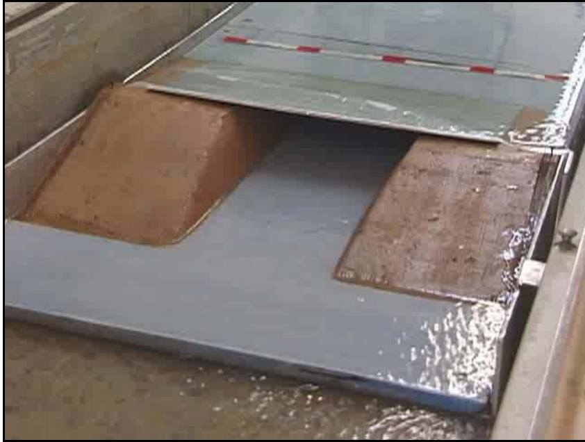
Figure 5.3. Test of a gated structure combined with a tarp showing almost no residual flow.
