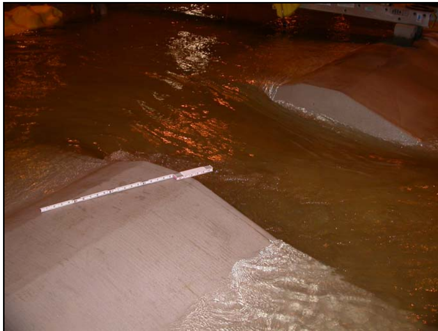
Figure 6.2. Flow through the breach with upstream depth at 18.7 ft.
