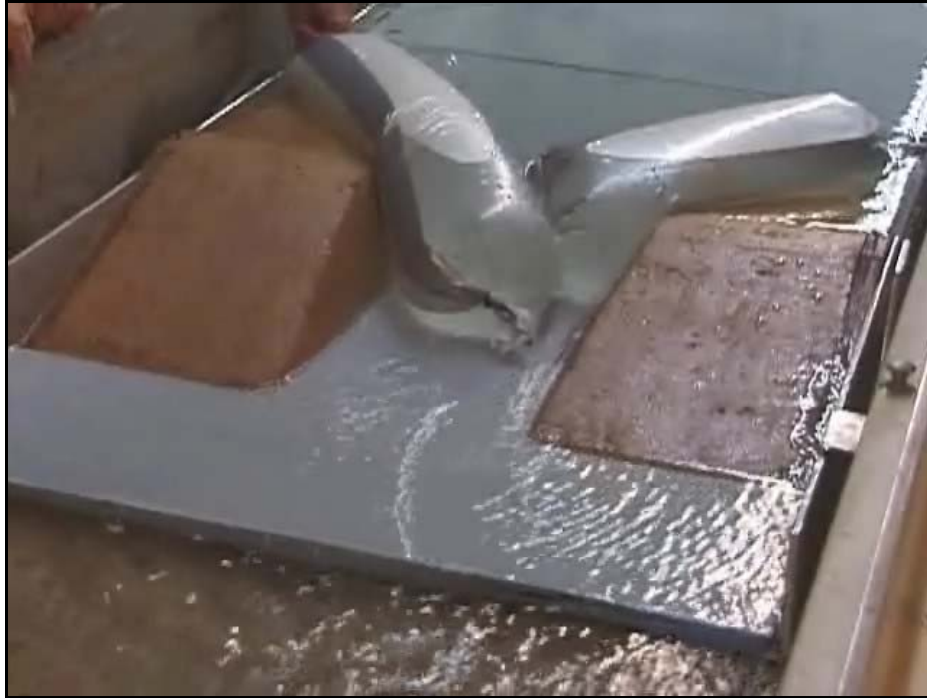
Figure 5.6. Photo of water-filled tube concept utilizing two tubes anchored to either side of a breach in the 1:50 scale model basin.
