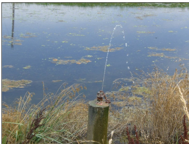
Figure K-7. Overflowing Piezometer.
