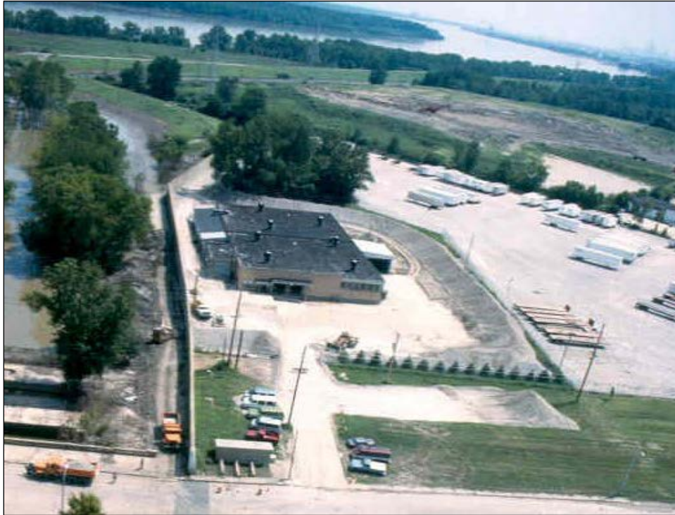
Figure K-18. Emergency Seepage Berm Between Flood Wall and Adjacent Building with Full Height Flood Barrier Constructed Landside to Prevent Flood Waters from Entering the Leveed Area through a Concentrated Leak Under Floodwall.
